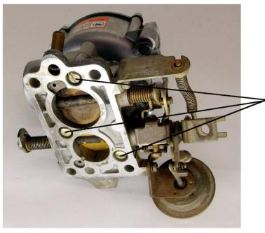
Use the 3 screws from the 22R gasoline carburetor
