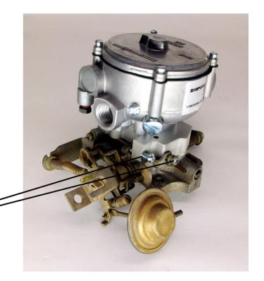
Remove three screws that hold the throttle plate to the carburetor
